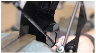
4. Cut off the bottom of the piece of the bracket that he saw is threded through. The cover should look like this:
