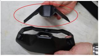
3. Next, thread the blade of the hand saw through the cover like the image below:
