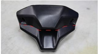
We recommend making two different cut lines. Start on either the right or left side and saw to the center of the cover. Remove the blade and then resume sawing from the other side so that the saw lines meet in the middle.
